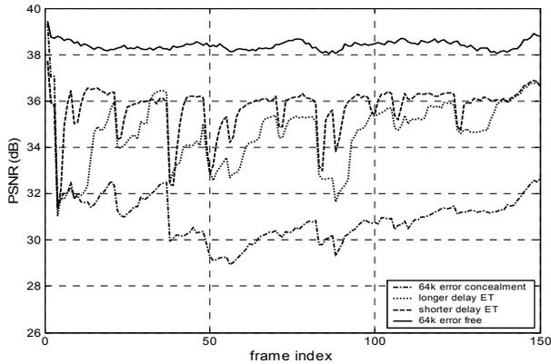
Fig.3 Error tracking improvement curves at a mean packet loss rate of 1%
