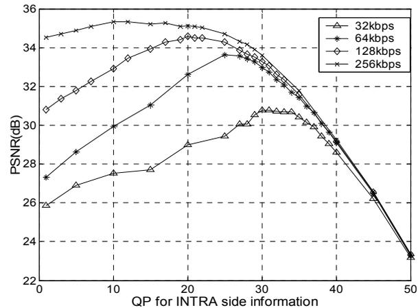
Fig.5 Best QP for different transmission rates at a loss rate of 5%
