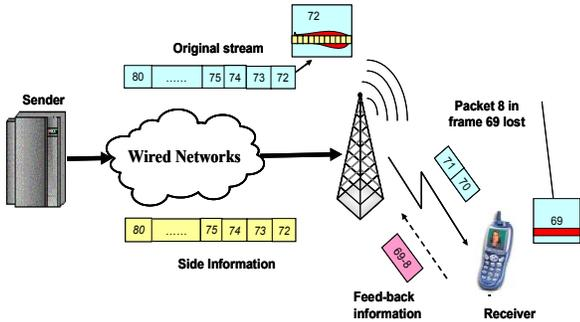
Fig.1 Proxy-based error tracking scenario
