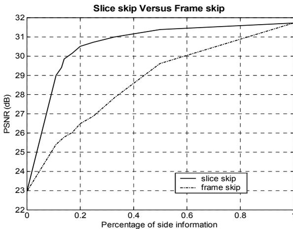
Fig.6 Performance of error tracking as a function of side information skipping rate at 10% packet loss rate
