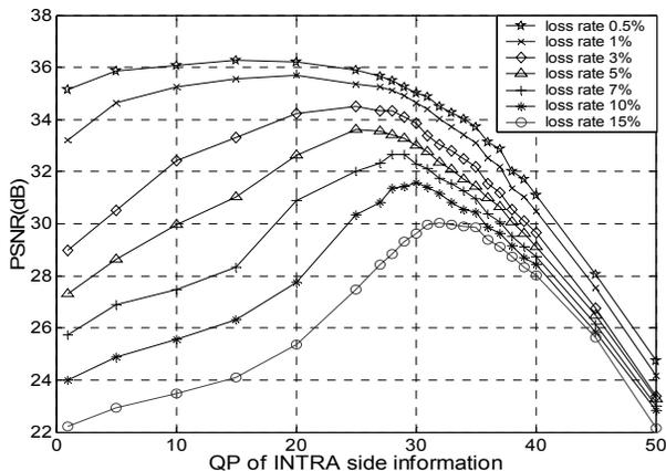
Fig. 4 Best QP for different loss rates in a 64kbps channel, QP of the original bit-stream is 27
