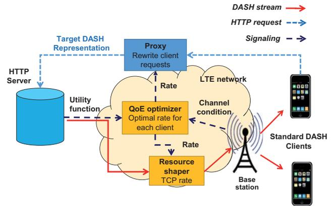
Fig. 1. QoE-Based adaptive HTTP system architecture [5]
