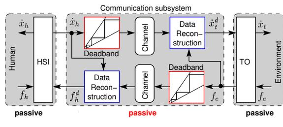
Fig. 2. Deadband controlled teleoperation system
