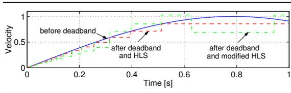
Fig. 3. Effect of deadband and data reconstruction
