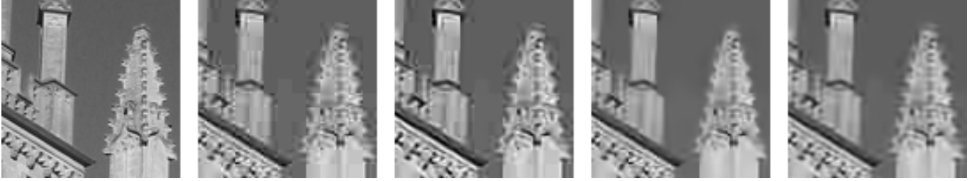
Fig. 1. From left to right: Original image, JPEG-encoded image with quality value 12 (PSNR = 28.4 dB), DIP deblocked image (PSNR = 27.8 dB), SA-DCT deblocked image (PSNR = 29.2 dB), REAPP deblocked image (PSNR = 28.9 dB).
