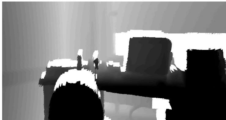
Figure 7: Triangulated geometry warped into a captured image (Part of Figure 5 - left). Darker areas are nearer to the camera.
