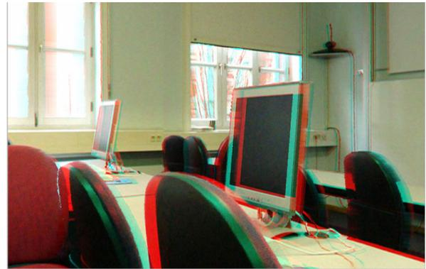
Figure 6. Perspective stereoscopic view rendered from a single viewpoint panorama with depth information (anaglyph).
