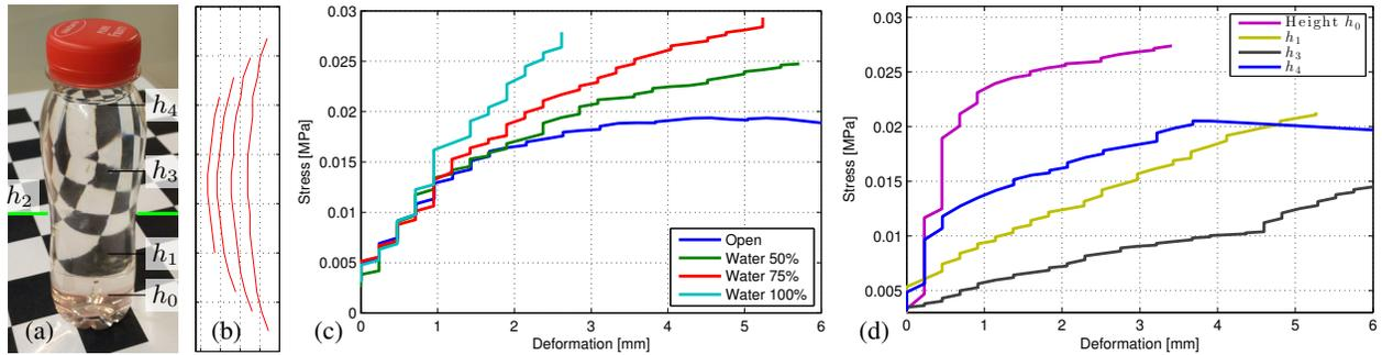
Fig. 2. (a) A transparent bottle (depicted in front of a chessboard pattern) is explored. Note the slight narrowing at half height ( $h_2$ , green line), which explains the low stiffness in this region. (b) Deformation shapes measured at the center of the bottle while increasing the pressure. (c) Stiffness at height  $h_2$  with open cap or closed cap and varying levels of water inside. (d) Stiffness varies considerably along the height of the bottle (measured with open cap).
