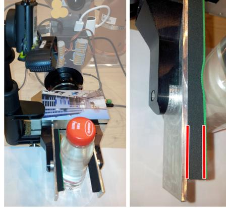
Fig. 1. *Left*: The proposed sensor consists of one or two low-cost webcams (top-left) and passive rubber foam strips on the fingers of a gripper (bottom). *Right*: Detailed view of the foam strip with its front painted in green. The deformation in the contact region at the center is measured visually using the camera. In the lower part, the red lines indicate the locations of the two contours tracked by snakes (reference and front).
