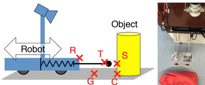
Fig. 1. For exploration, the robot pushes the sensor tip  $T$  onto an object. A camera tracks points on the robot and the scene (red, see text) to measure applied forces and the reaction of the object. Right: The pose of two sensor tips is obtained by tracking arbitrary templates (e.g. the Lenna image).
